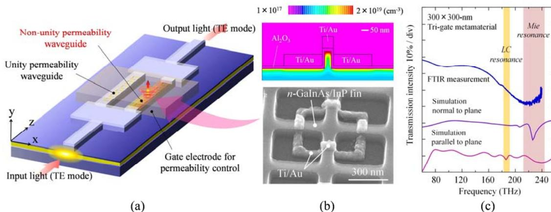
Fig. 1 (a) Permeability-controlled optical modulator consisting of InGaAsP/InP Mach-Zehnder interferometer with Tri-gate metamaterials. (b) SEM image of TGM unit cell (lower). Electron densities in the fin at  $V_g = 10$  V, calculated by 3-dimensional TCAD simulation (upper). (c) Normal-incidence transmittance spectra for 300×300 nm TGM.
