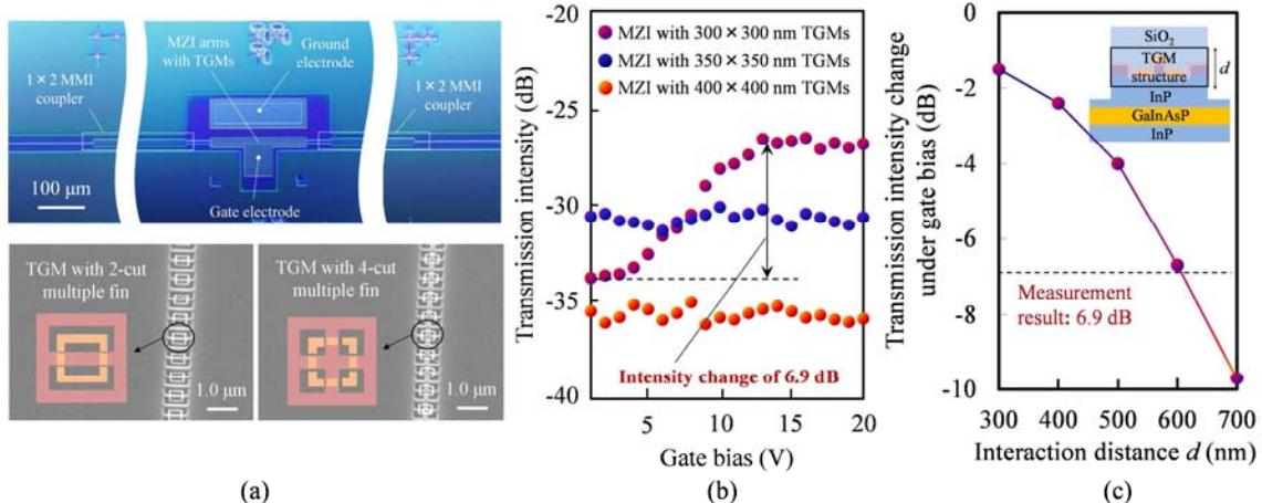
Fig. 2 (a) Plan-view optical microscope image of the permeability-controlled optical modulator (upper). Oblique view of TGMs for MZI arms, observed with SEM (lower). (b) Transmission characteristics of the device as a function of gate bias, measured for 1550-nm TE-polarized light. (c) Transmission intensity change of the device as a function of an interaction distance of the TGM, calculated by finite difference methods.
